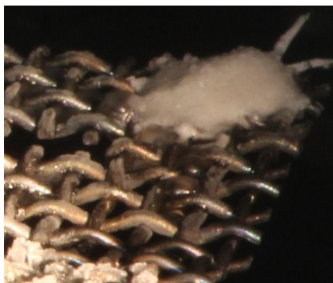
Figure 33: Picture of discolored, bubbling HAN under heated conditions
